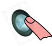
The pendant button will **FLASH RED ((••))** for several seconds after the button is pressed.
